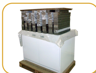
Actual photo during Cabinet Load Testing
